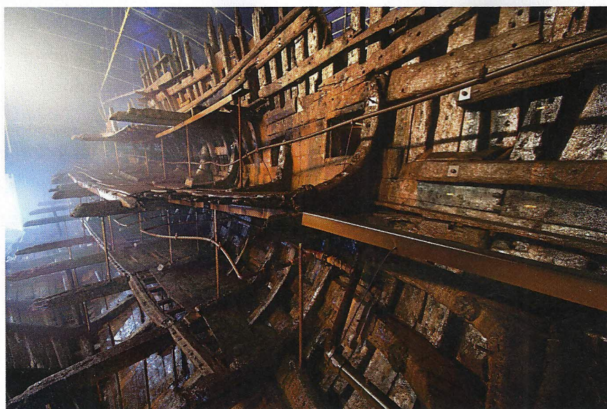
Fig.2. Interior of hull during preservation process using PEG
